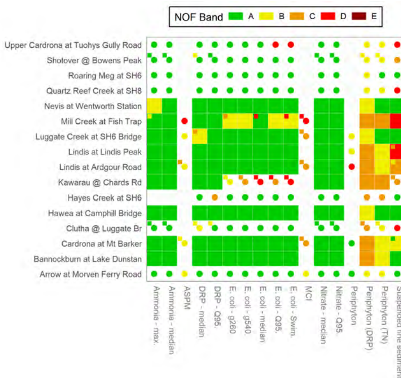
Figure 10 Grading of the river sites of the Dunstan Rohe based on the NOF criteria. Grades for sites that did not meet the sample number requirements in Table 1 are shown as white cells with coloured circles. The white cells indicate sites for which the variable was not monitored. Small square in the upper left quadrant of the cells indicate the site grade for the baseline
