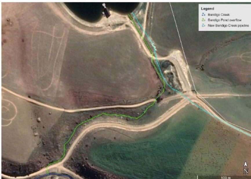
Figure 10: Annotated aerial photograph showing flow path from Bendigo Station pond to Bendigo Creek via the spillway. Source: Application.
