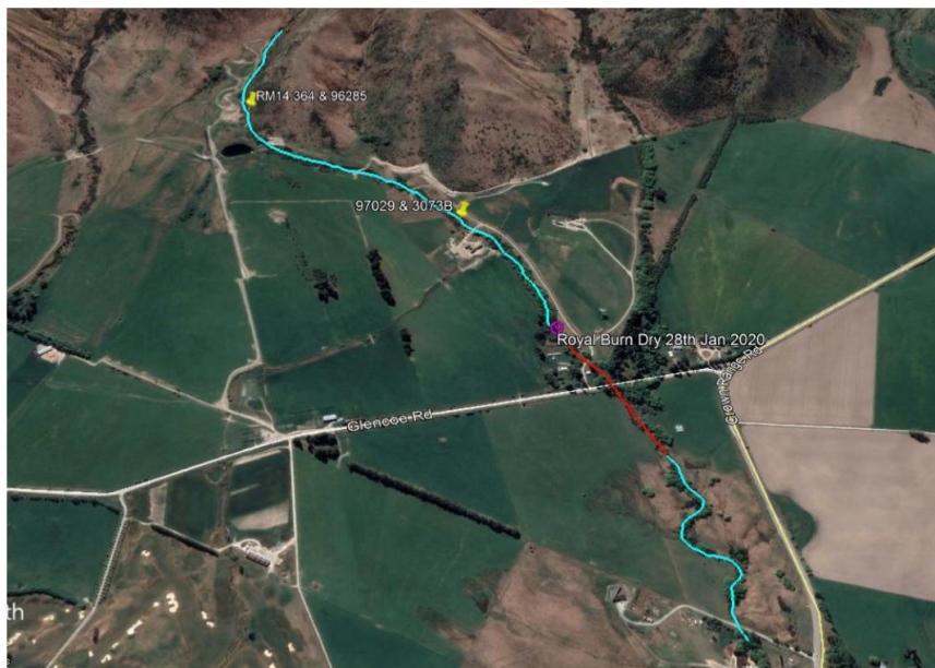
Figure 4. Map showing the flow reaches of the Royal Burn (blue line) the dry reach (red line) and the point the North Branch went dry despite the majority of flow passing the intake for 97029 & 3078B.
