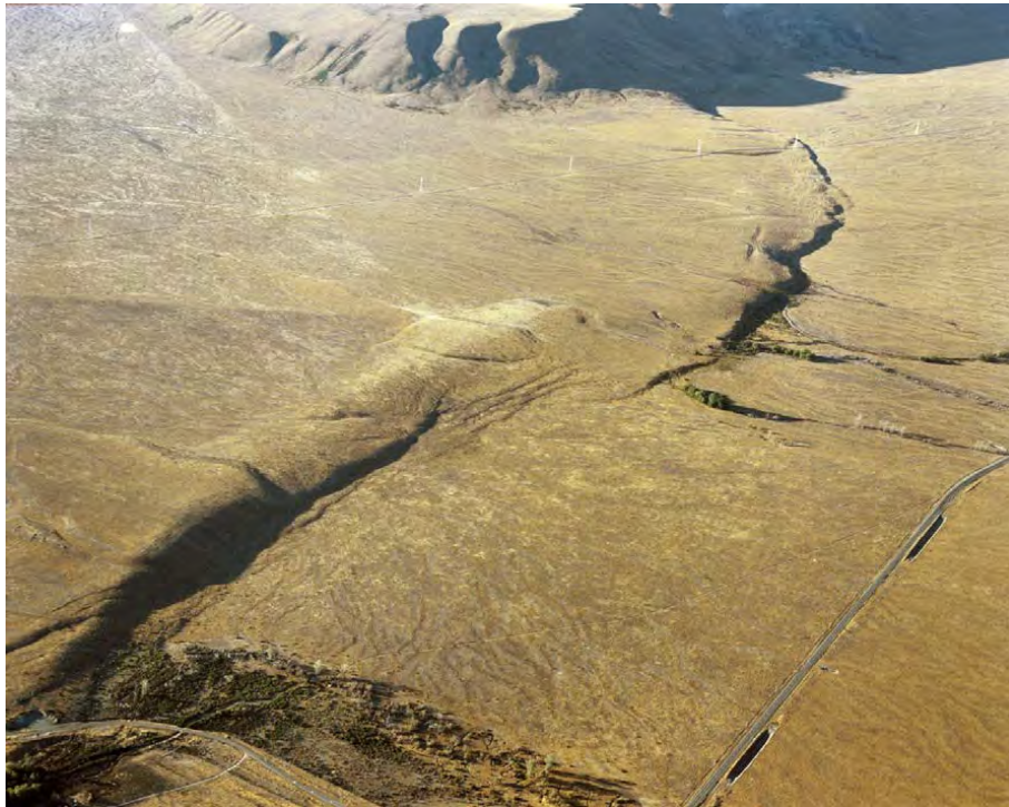
Figure 1.3 A northward oblique aerial view of ground-surface deformation across the Ostler Fault Zone, in the Waitaki District in the Canterbury region, about 12 km southwest of Twizel. The fault zone runs from lower left to upper right and has offset and buckled a ~22,000-year-old glacial meltwater outwash plain with well-preserved relict braided channels. This location is one of the best expressed examples of fault deformation in New Zealand because it is entirely across old landforms. This view shows complicated elements of main and subsidiary fault offsets and folds across a zone that is several hundreds of metres wide. All of these elements form part of a single entity, the Ostler Fault Zone. This figure is taken from Barrell (2016), where a more detailed description of the features in this view is provided. Photo: GNS Science, CN576/B and VML ID: 5151. DL Homer, taken 1995.
