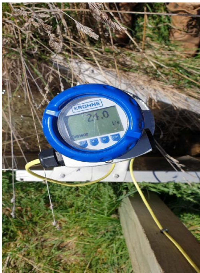
Figure 2: Flow Measurement on 28 October 2020 Parshall Flume
