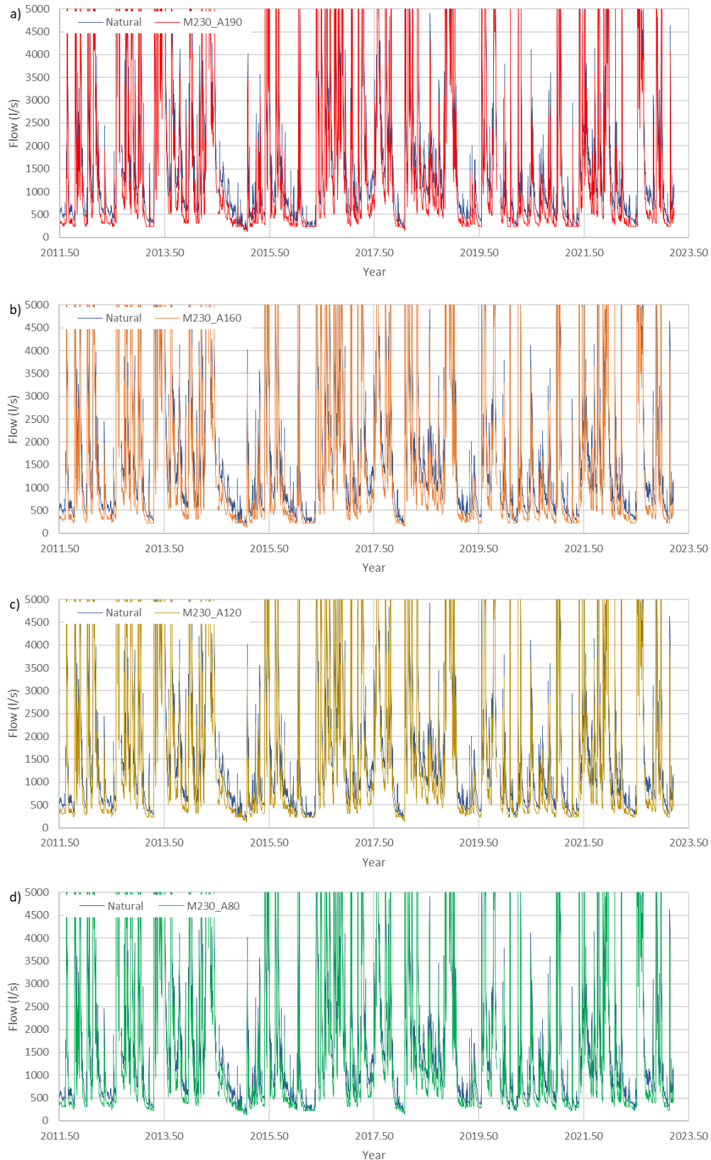
Figure 15 Hydrographs of allocation scenarios with a minimum flow of 230 l/s. a) Current allocation limit 190 l/s, b) allocation limit of 160 l/s, c) allocation limit of 120 l/s, d) allocation limit of 80 l/s.
