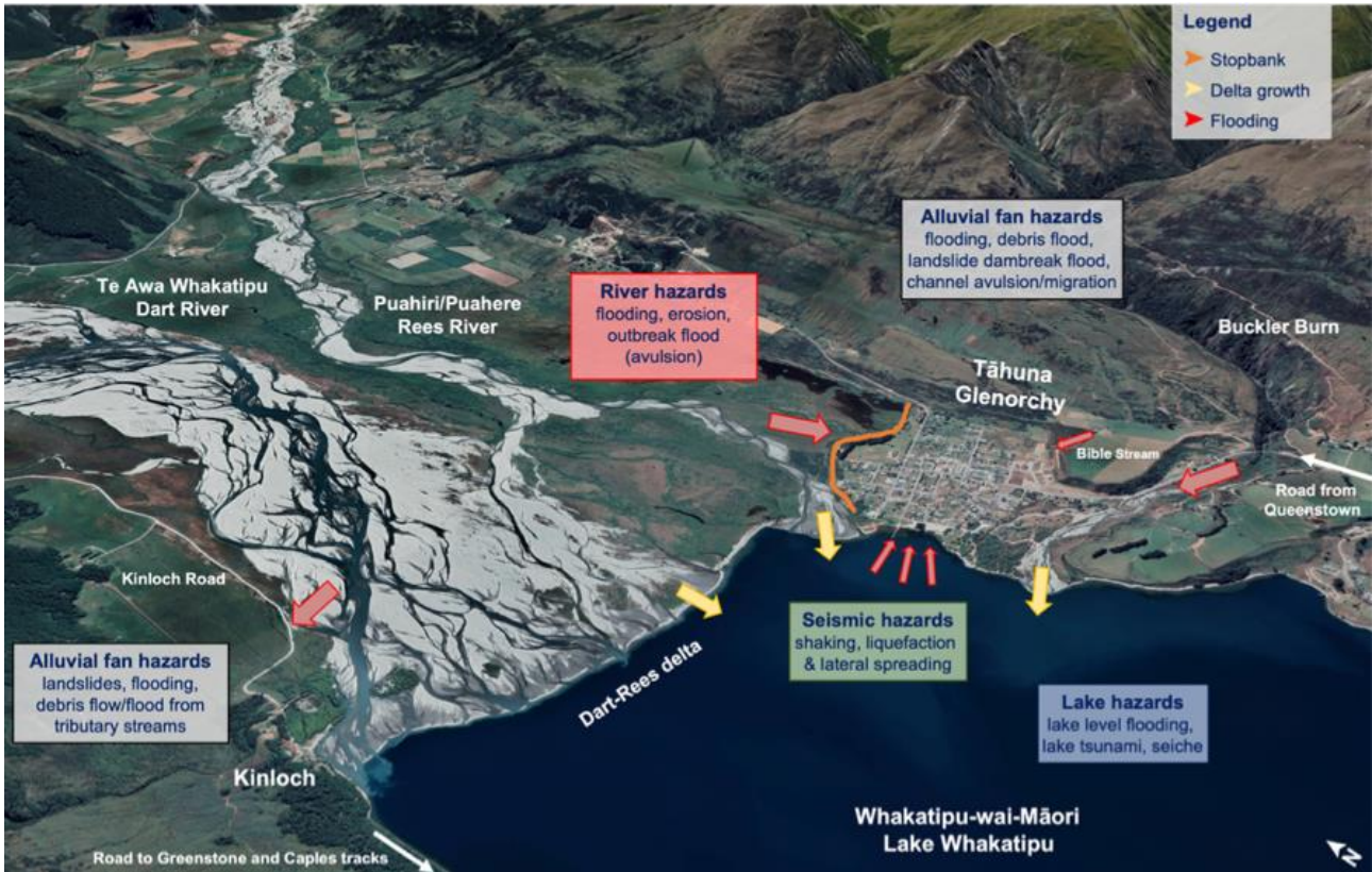
Figure 6-1: Head of the Lake natural hazardscape. Source: (MacKenzie, 2023)
