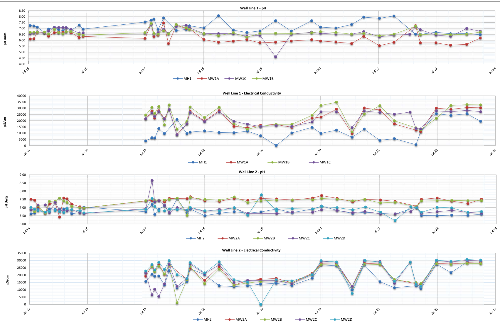
Figure C3-1: Green Island Landfill - Manhole, Shallow Monitoring Wells and Pump Station pH and EC Data
