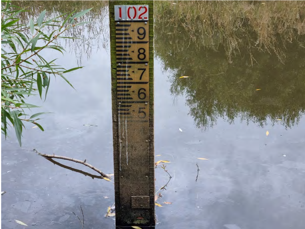
Photograph 13: All staff gauges require cleaning to make the numbers and ticks legible.
