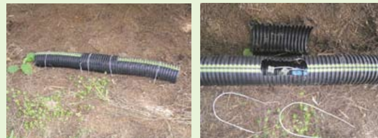
Figure 4. A 1 m-long, 100 mm-diameter draincoil rodent bait station secured to the ground with No. 8 wire (left). Internal spikes secure Ditrac and Storm anti-coagulant poison blocks (right).
